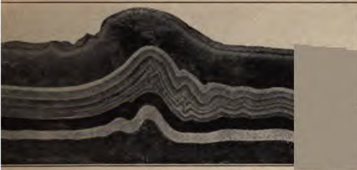
layers compressed in experiments and showing the effect of a competent layer in the process of folding (after Willis).
